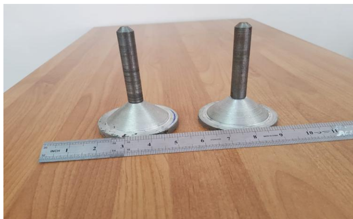
Picture 1. Models of conical foundations with a rack and changing in area by the console heel
