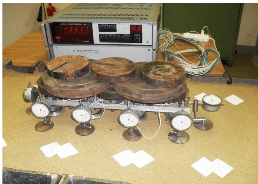
Figure 1. Testing of a strain gauge beam on truncated conical foundations
