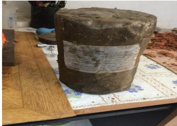
Figure 1. A sample of soil sample (monolith)
