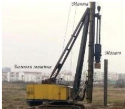
Figure 2. Diesel hammer
