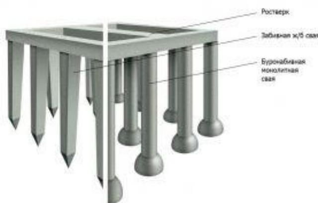
*Figure 1. The scheme of pile foundation*
